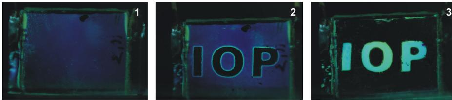
Fig. 5. The photoinduced inversion of optical images in CLC cell with homeotropic anchoring. The 10  $\mu\text{m}$  cell based on non-rubbed SE1211 alignment layers and filled with CLC MLC6884/PBM/R811 is viewed between crossed polarizers (picture 1). At first the cell is irradiated during 40 s through a mask with the transparent areas in an “IOP” form (picture 2) and then during 40 s entirely (picture 3). As a result, image 3 is inverted to image 2.
