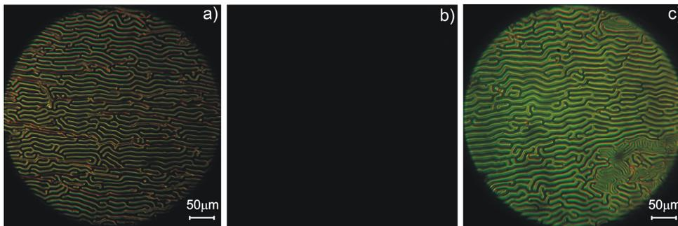
Fig. 3. Microphotographs corresponding to areas 1, 2 and 3 in Fig. 2; (a) fingerprint texture of a left-handed cholesteric LC, (b) compensated nematic texture, and (c) fingerprint texture of a right-handed cholesteric LC.
